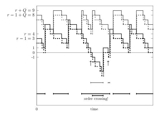
Figure 1: A comparison of policies  $\pi(r,Q)$  and  $\pi(r-1,Q)$  for r=4 and Q=5. The (remaining) lead time realizations and demand realizations are chosen arbitrarily.
