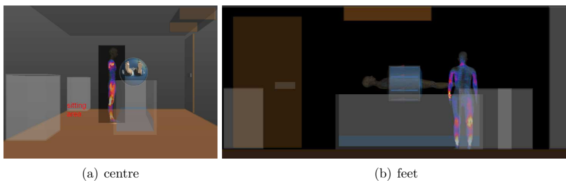
Figure 11.6: Localized specific absorption rate ( SAR_{10g} ) distributions in medical staff for standing near the centre of the applicator or near the feet of the patient. The colorscale is from black (0%) to white (100%)
