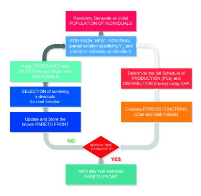
Figure 2: Schematic flow chart of the MOGM.
