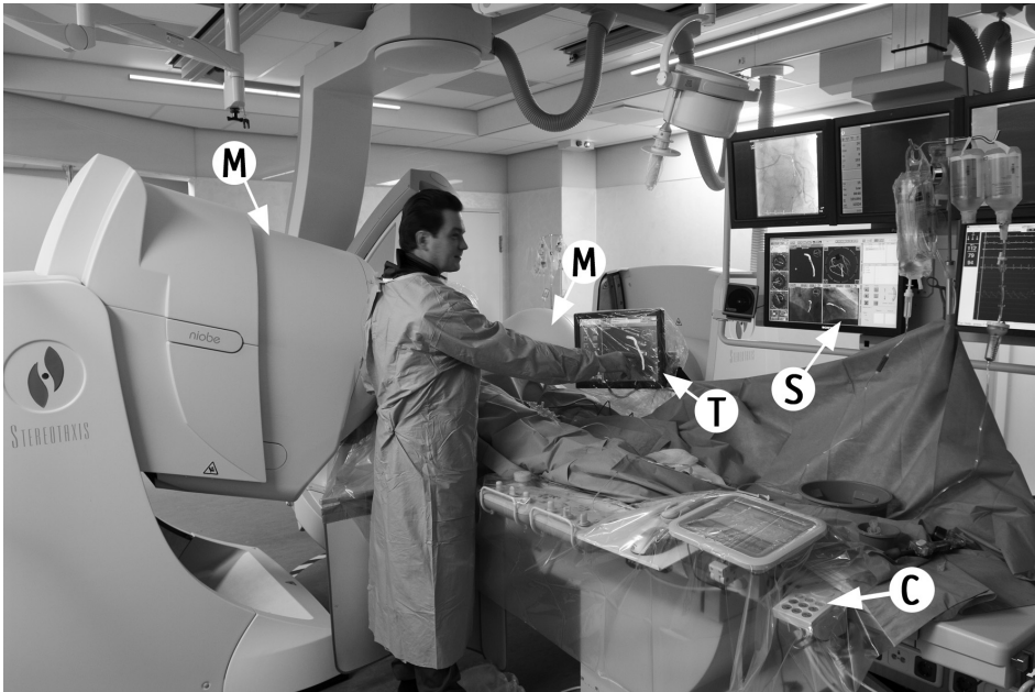
Figure 1 The Niobe® Magnetic Navigation System in position for PCI. M indicates magnets in tilt position for better lateral movement of the image intensifier. T indicates touch screen interface to give real-time instruction to the MNS. S indicates in-lab main screen monitor, C indicates the controls for magnet deployment. See this figure in color in the Appendix page 394.
