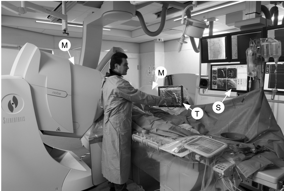
Figure 1. System in position for PCI. M indicates magnets in tilt position for better lateral movement of the image intensifier. T indicates touch screen interface to give real-time instruction to the MNS. S indicates in-lab main screen monitor. See this figure in color in the Appendix page 378.
