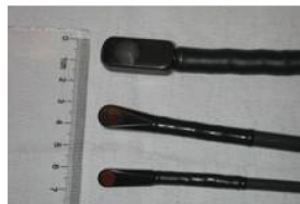
Figure 6.1: Photograph of the new probe (micro-multi) together with 2 commercially available TEE probes. Top: Adult probe, Middle: mini multiplane probe, Bottom: micro multiplane probe.
