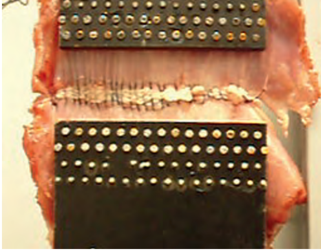
Figure 1 Photograph of the test setting used. The sutured abdominal wall is fixed in the tensile testing machine and is pulled apart at a constant rate of 10 mm/min.
