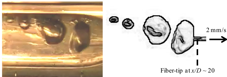
Fig. 6. Left: photograph of vapor bubbles occurring in water with a bare tip at 2 mm/s and relatively high laser power (25 W). Right: schematic showing the biggest bubbles as well as the position of the fiber tip.
