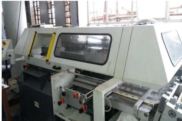
Figure A6.2 Photo Narration - Perfect Binder Printer
