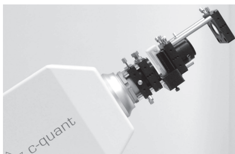
Figure 3. Adaptation of the C-Quant to evaluate straylight from IOLs.
