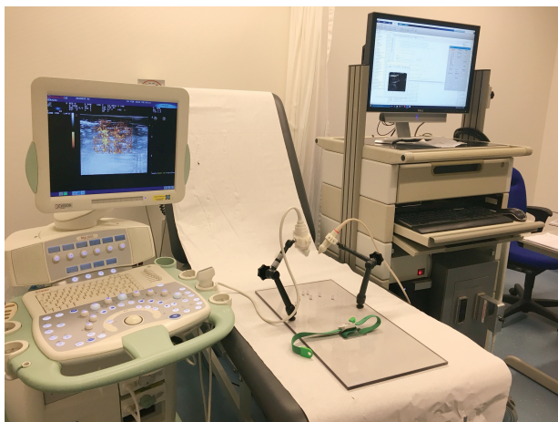
Figure 2. Experimental set-up for the proof-of-principle study with the probe-mounting arms and the custom plate with pins to spread and fixate the fingers. Left machine: Esaote MyLab 60; right machine: Verasonics Vantage-256 on a custom trolley.
