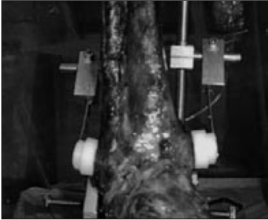
Figure 2 Malleolar clamp with strain transducers.
