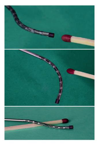
**Figure 4.2** Multisteerable Tip of *Accura* illustrating different curvatures. Top: Complex single-plane curve side view. Middle: Single-plane 90° single-radius curve top view. Bottom: Complex 3D-curve side view. The match is illustrated for scale purposes.
