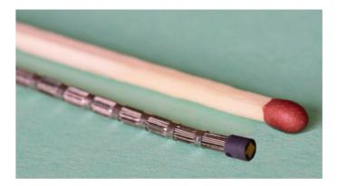
Figure 4.6 Catheter steerable tip and single-element transducer compared to a match.
