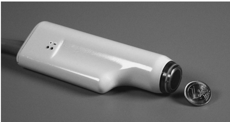
Figure 1: Latest prototype of the continuous fast-rotating transducer.
