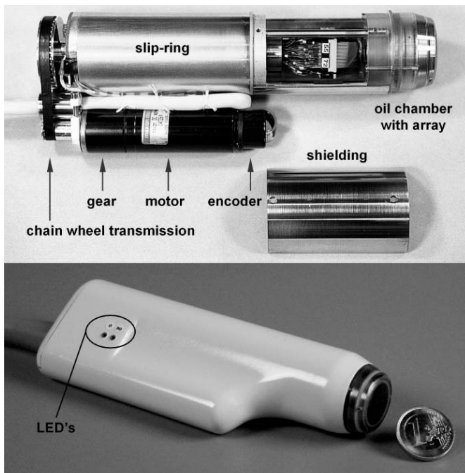
Figure. 1. The latest prototype of the fast-rotating ultrasound (FRU)-transducer. The upper panel shows the construction of the transducer with some key components annotated. The lower panel shows the transducer with its housing. Note the LEDs on the housing, which are used to indicate whether the phased array is located in one of its two fixed positions ( 0^\circ and 90^\circ ).
