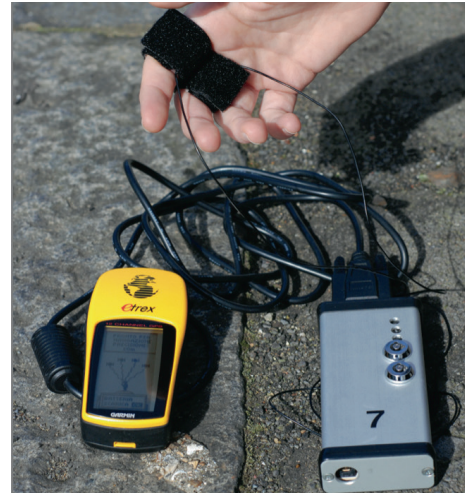
Figure 3.5: “The Bio Mapping device: GPS - left, finger cuffs - top and data logger on the right” (Nold, 2009, p.3)
