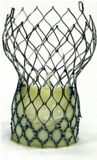
Fig. 14.2 The first generation CoreValve ReValving System bioprosthesis housing trileaflet bovine pericardial leaflets. The current third generation Medtronic CoreValve bioprosthesis houses leaflets made of porcine pericardium.
