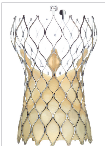
Figure 1 The CoreValve Evolut R. The CoreValve Evolut R has been redesigned to provide more consistent radial force across the sizing range with modified cell geometry to improve conformability to the aortic annulus. The new valve release mechanism has a paddle design to prevent hang-ups and the porcine pericardial leaflets are treated with alpha-amino oleic acid (AOA®) to retard mineralisation.
