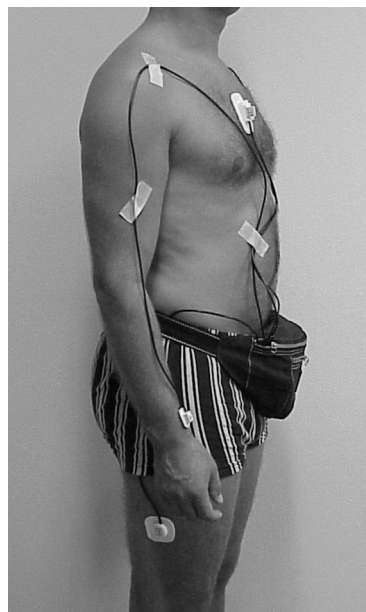
Figure 5.2: A subject wearing the Upper Limb-Activity Monitor.
