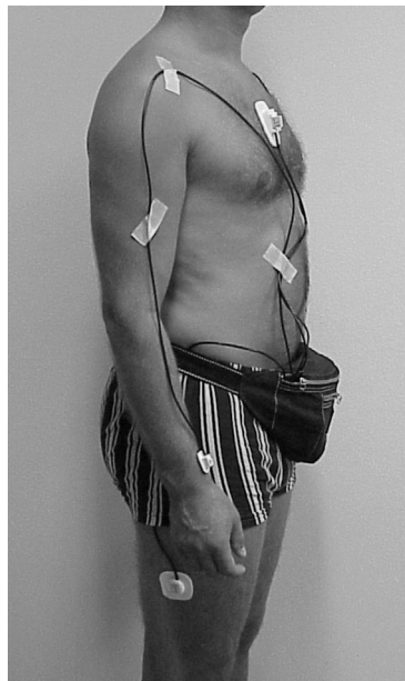
Figure 5.2: A subject wearing the Upper Limb-Activity Monitor.
