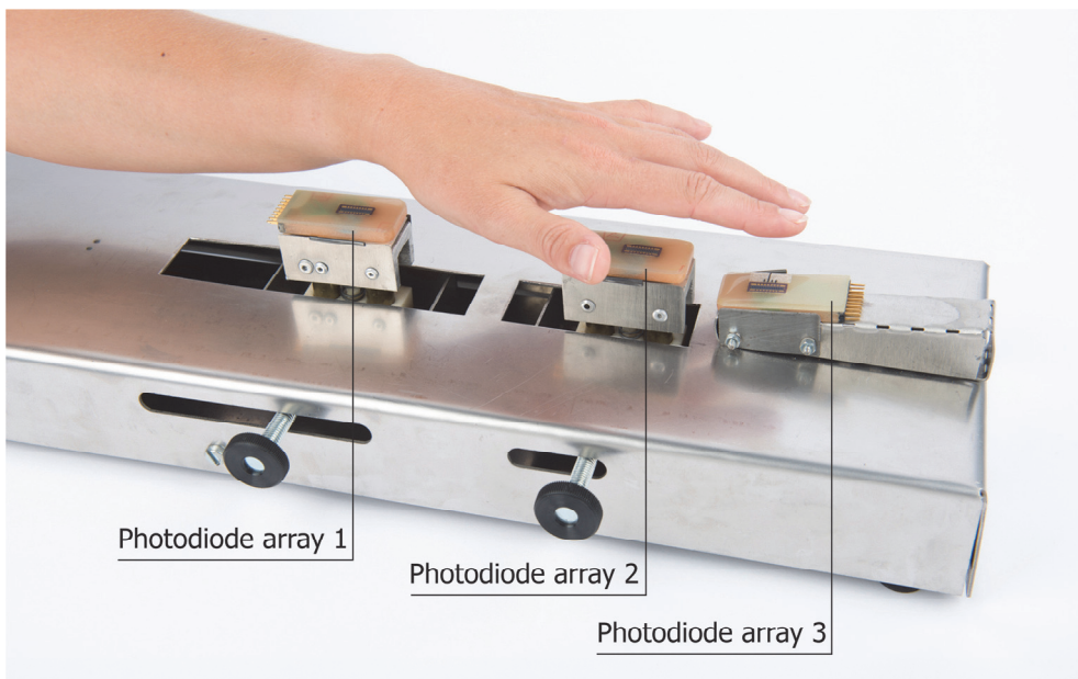
Figure A.4: The smart sensor holder with the fingertip, wrist and lower arm each lying on one of the three MPA-sensors.
