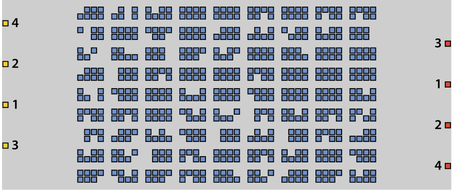
Figure 4.6.1: Top view of the small layout, including station activation sequence numbering, with the storage area in the middle, replenishment stations to the left, and pick stations to the right
