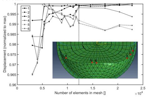
**Supplemental figure 5.1:** Results of the mesh convergence study. The absolute maximum displacement of the node, normalised to the maximum between meshes, is shown on the y-axis. The number of elements is shown on the x-axis. The colours correspond to the different nodes. The chosen mesh has 12288 elements in the vitreous (see dotted line).
