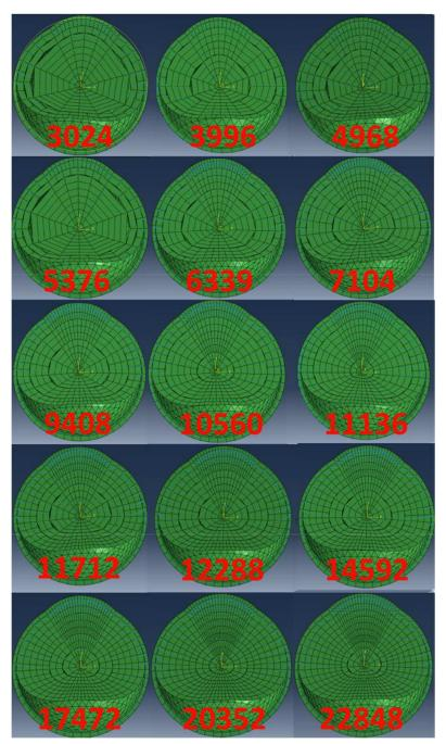
**Supplemental figure 5.2**: All iterations of the mesh convergence study. Shown in red are the number of elements of the vitreous. The "gaps" between some of the elements are an artefact and are not present in the nal calculation of these models.
