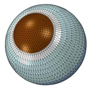
The next set of three layers, towards the center, consist of 16 rings of elements and the three innermost layers consisted of eight rings of elements. The center was filled with 192 tetrahedral elements to fill the remaining space. The elements were attached to the adjacent elements using a tie constraint. See Table 1 for an overview of all elements in the model.
