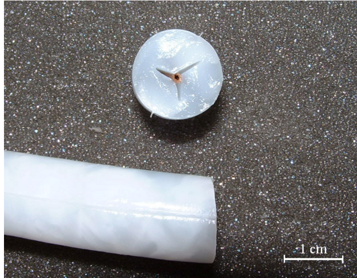
Figure 2.3: Cross section and side-view of a PVA model urethra (reproduced from NeuroUrol. Urodyn. 24(4): 381-388, 2005, with kind permission of John Wiley & Sons, Inc.).
