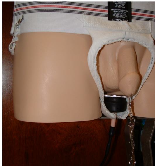
Figure 8.2: Modified jockstrap to fix the microphone at the perineum during voiding.
