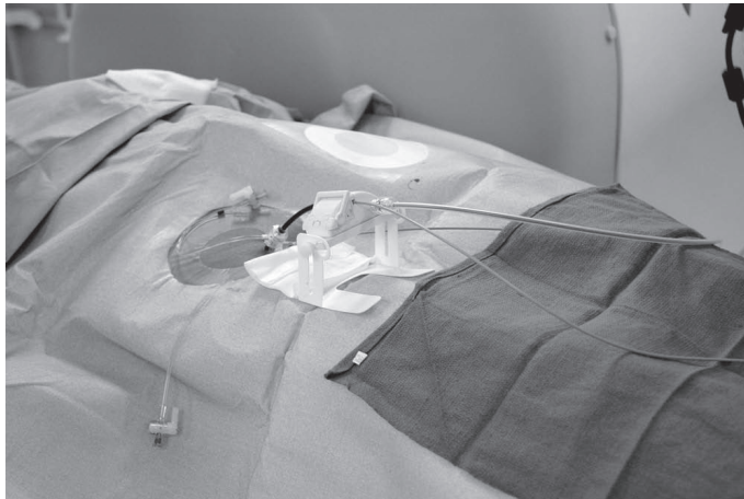
Figure 1 The catheter advancer system (Cardiodrive) is placed on the anterior thigh and used remotely to advance and retract the catheter. It uses a simple cogwheel system and is driven by a fixed rate motor attached via a flexible drive cable. An adaptor between the Cardiodrive and the sheath prevents buckling of the catheter.
