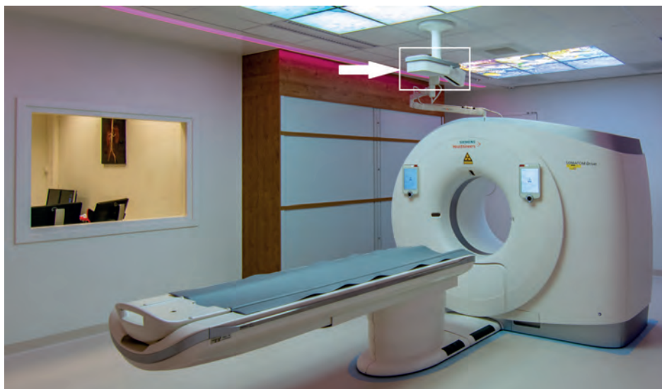
Figure 3. 3D camera for body contour detection (white arrow and box) positioned above a dual source CT scanner of the Erasmus MC University Medical Center Rotterdam.
