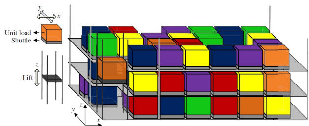
Figure 2.14: A Live-Cube storage system with lift (Zaerpour et al., 2015)
