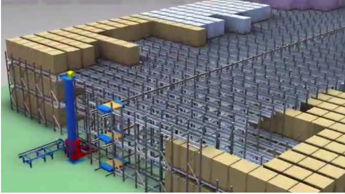
Figure 2.10: Multi-deep shuttle-based compact storage system (Tappia et al., 2016)
