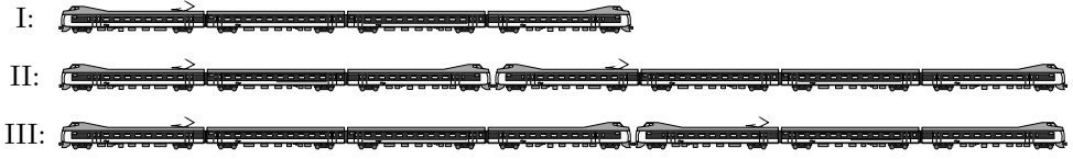
Figure 5.1: Example of three compositions comprised of ICM-III (3 carriages) and ICM-IV (4 carriages) train units. Note that the train units in the last composition are in reversed order compared to the second composition.
