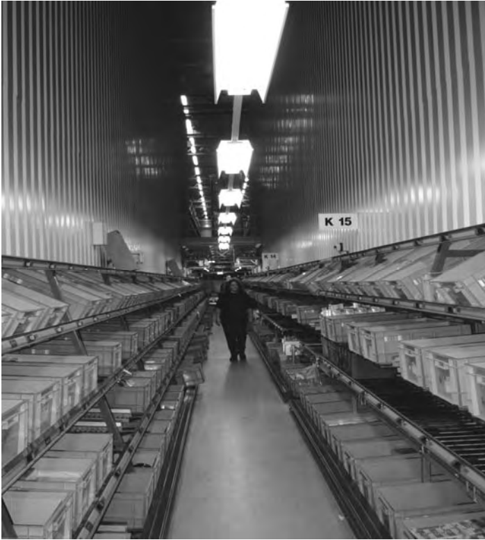
Figure 4.1: An illustration of a DSS at Nedac Sorbo : the S/R machines replenish the pick bins from a bulk storage area behind the walls.
