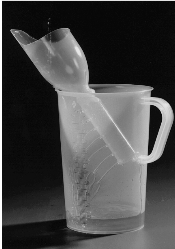
Figure 6.2 A self-made prototype of the low cost flow meter with the dimensions of experimental model 2 (see table 6.1) to grade the maximum flow rate. The funnel and collecting tube are placed in a measuring cup to measure the voided volume.
