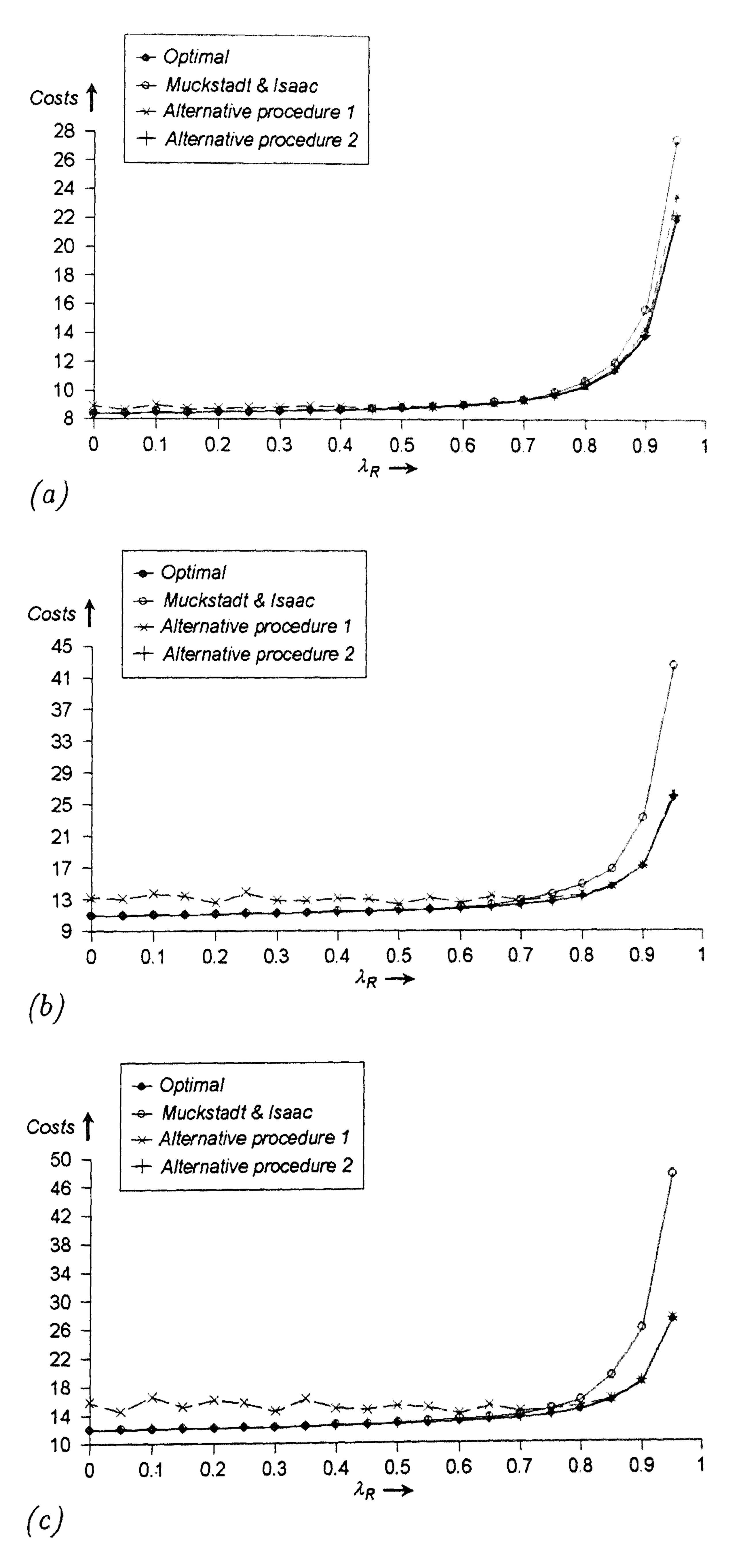
Figure 7.1 Exact expected total costs as function of the return intensity, under the optimal strategy and under the strategies determined by the approximation procedures, with  $c_b = 10$  (a),  $c_b = 50$  (b), and  $c_b = 100$  (c).
