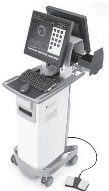
Figure 1: the mobile OCT cart incorporating the system console, monitor, and patient interface unit
