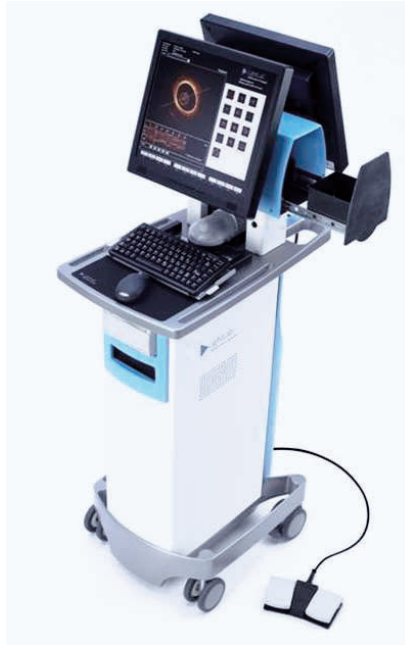
Figure 1: the mobile OCT cart incorporating the system console, monitor, and patient interface unit
