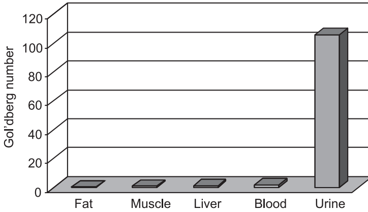
Figure 2.3: Gol'dberg number calculated for different media at a transmit frequency of 3 MHz and acoustic pressure of 1MPa
