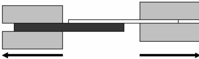
Figure 1. Tensile strength of the tissue that adhered to and incorporated the mesh was measured on a dynamometer
