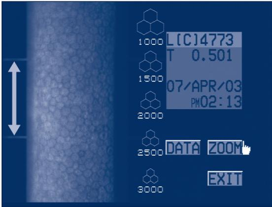
Figure 3.1b Picture of external microgrid used with calibration device as it appears on the SP-2000P screen. The double headed arrow indicates the mask slit width. The distance between lines A and B is a standard distance used to calculate the mask slit width.
