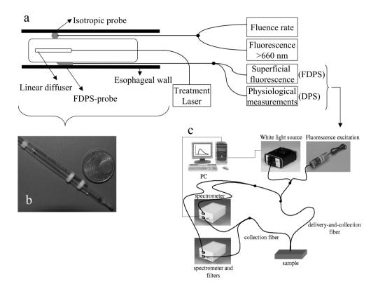
Figure 1. a) Shows a schematic diagram of the experimental setup; b) Photo of the balloon with the isotropic and DPS probe attached to the balloon; c) schematic diagram of the FDPS system.
