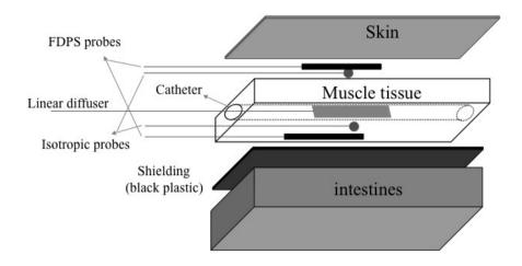
Figure 1. Schematic detailed outline of the placements of the linear diffuser to deliver the treatment light to the tissue, and the measurement probes (FDPS and isotropic probes) on top and bottom of the muscle tissue.
