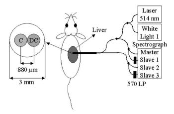
Figure 1. Schematic diagram of the FDPS measurement setup. The probe tip with a diameter of 3 mm contains two 800 μm fibers at a core-to-core distance of 880 μm.
