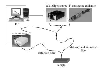
Figure 1. Schematic diagram of the FDPS setup.
