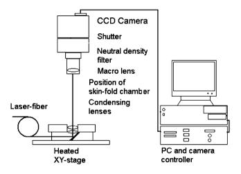
Figure 1. The schematic diagram of the setup
