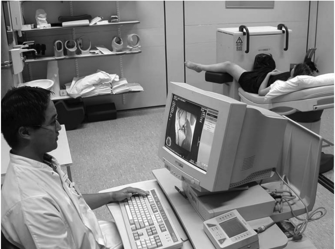
Figure 1. Design of the Artoscan M (Esaote Biomedica, Genoa, Italy) low-field dedicated extremity MRI scanner.
