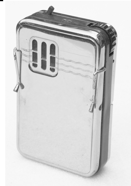
Figure 4-0: Audium model 600. Body-worn hearing aid with three miniature electron tubes (made by Hivac) and built-in microphone. This example dates from around 1950. Dimensions 9.2x5.7x2.1 cm. Two batteries are needed for operation: 45 Volt for the plate voltage and a 1.5 Volt cell for heating of the filaments. Circuit diagram reconstructed by the author. Hearing aid from the author's collection. Photograph by the author.
