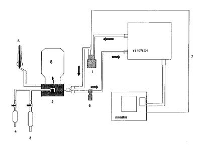
1=humidifier 2=burner unit 3=gas tank 25 ml (stabilization prior to experiment) 4=gas tank 10 ml (experiment) 5=test lung 6=water trap 7=inspiratory gas sampling line 8=Pyrex glass jar
