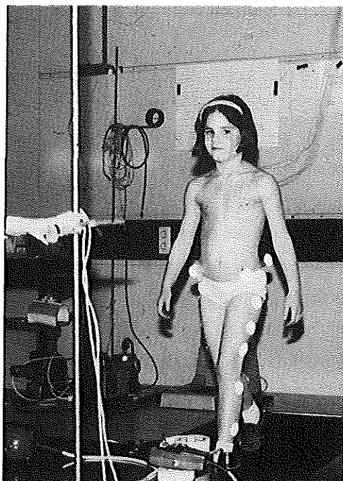
Figure 3.1 A child with infrared reflecting markers on the treadmill, with permission.
