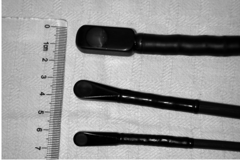
Figure 1: Photograph of the new probe (micro-multi) together with 2 commercially available TEE probes. Top: Adult probe. Middle: mini multiplane probe. Bottom: micro multiplane probe.
