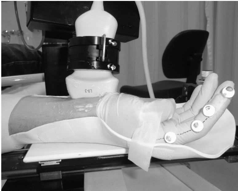
Figure 1. Experimental conditions with the subject's arm positioned in the custom-made brace. Four markers on the index finger were used to automatically track the joint angle.
