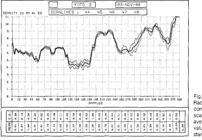
Fig. 10a, 10b. Radiograph and computer-generated scan showing the average Al. eq values/mm<sup>2</sup> and the standard deviation.
