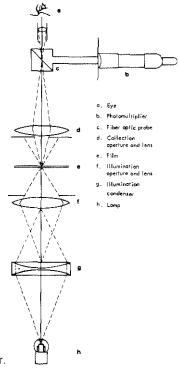
Fig. 6. Schematic drawing of a microdensitometer.
