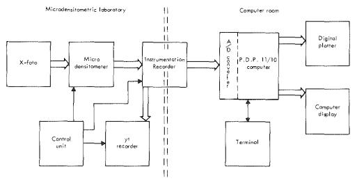
Fig. 9. Diagram of computing facility and microdensitometric laboratory.
