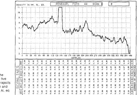
Fig. 17. The spread of five identical trajects of 0.2 mm and the mean Al. eq values.
