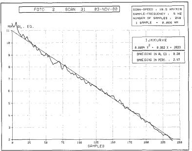
Fig. 3. The quadratic curve-fit shows the Al. eq values (11 - 2 mm Al.) the straight line indicates the real Al. eq values, the curved line shows the Al. eq values of the wedge as computed according to the quadratic formula from the registered data.
