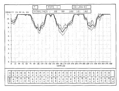
Fig. 25. Example of the spread of five horizontal trajects of 0.2 mm and the average value (mean) in one radiograph. The mean Al. eq value over a scan length of one mm (15 samples) and the standard deviation of the five scans is given.
