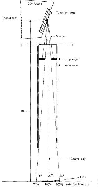
Fig. 5b. The heel-effect as given in the literature adapted to the long-cone technique (ref. The Fundamentals of Radiography).
