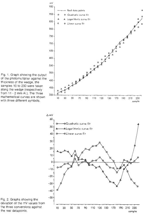
Fig. 1. Graph showing the output of the photomultiplier against the thickness of the wedge, the samples 10 to 230 were taken along the wedge (respectively from 11 - 2 mm Al.). The three mathematical curves are shown with three different symbols.
