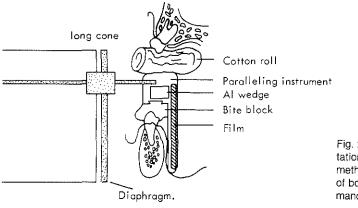
Fig. 23. Schematic representation of the radiographic method for the estimation of bone density in the mandible. The film was placed parallel to the axis of the teeth and the patient was asked to hold the biteblock in place with a finger. A cotton roll was sometimes used to secure the relationship object-film (fig. 23.).
