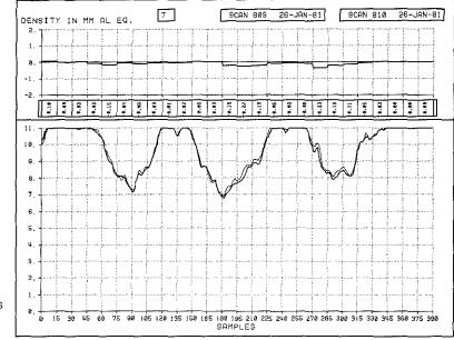
Fig. 27. Example of two scans illustrating the mean Al. eq values of two radiographs made during different sessions (interval of three months).
