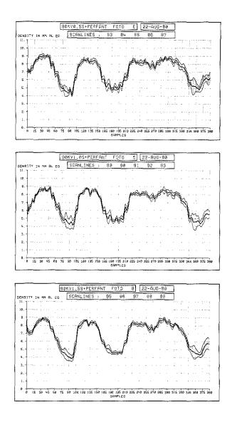
Fig. 16. Mean Al. eq value of the five scans and the standard deviation are shown. A one mm section of the curve track (sample 180 to 195) is evaluated in table IX.
