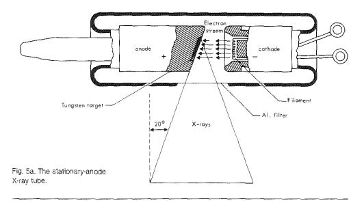
The inclination of the target gives a significant decrease in the intensity of the X-rays from the cathode towards the anode (heel-effect) (fig. 5a., 5b.).
