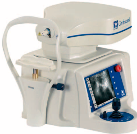
Figure 2. For the studies presented in this thesis, we used a slit scanning confocal microscope (Confoscan 4, NIDEK Technologies, Albignasego, Padova, Italy; reprinted with permission) equipped with a 100 watt halogen light source. Using a 40X Zeiss Acroplan objective lens with a high numerical aperture of 0.75, this instrument achieves a lateral resolution of 0.6 \mu\text{m}^1 and an axial resolution of 10 to 26 \mu\text{m} . 34,35 An optical coupling agent is applied to the objective lens to provide high-resolution images of 425 \times 320 \mu\text{m} , after reducing the blink reflex with topical anesthetics. A z-ring adapter can be used to further reduce the motion artifacts induced by involuntary eye movements, pulse, and respiration during the 12 seconds of image acquisition.
