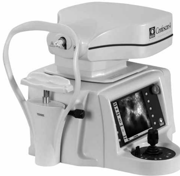
Figure 2. For the studies presented in this thesis, we used a slit scanning confocal microscope (Confoscan 4, NIDEK Technologies, Albignasego, Padova, Italy; reprinted with permission) equipped with a 100 watt halogen light source. Using a 40X Zeiss Acroplan objective lens with a high numerical aperture of 0.75, this instrument achieves a lateral resolution of 0.6 \mu\text{m} and an axial resolution of 10 to 26 \mu\text{m} . 34,35 An optical coupling agent is applied to the objective lens to provide high-resolution images of 425 \times 320 \mu\text{m} , after reducing the blink reflex with topical anesthetics. A z-ring adapter can be used to further reduce the motion artifacts induced by involuntary eye movements, pulse, and respiration during the 12 seconds of image acquisition. (See also Color figures, p. 203.)
