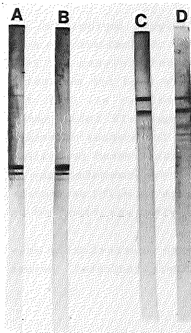
Fig. 5.1. Analytical isoelectric focusing in polyacrylamide gels of apolipoproteins in a pH gradient from 4-6.
