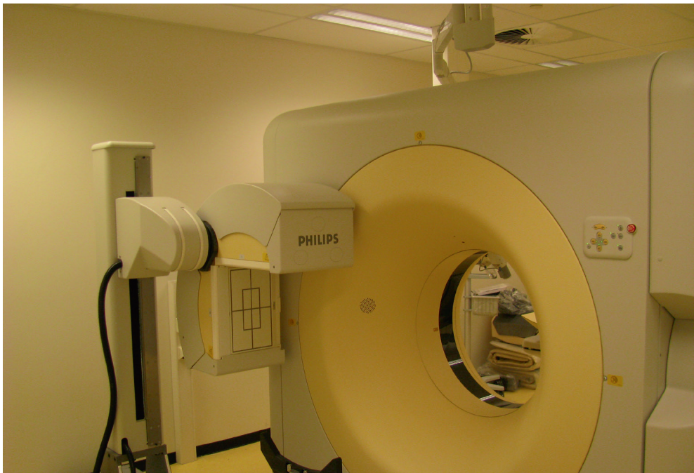
Figure 2 Hybrid SPECT-CT system, CardioMD gamma camera in the front and Brilliance 64-slice CT scanner in the back (Philips Medical Systems, Best, The Netherlands). The components share a common table (not in the picture) that is aligned to allow sequential image acquisition.
