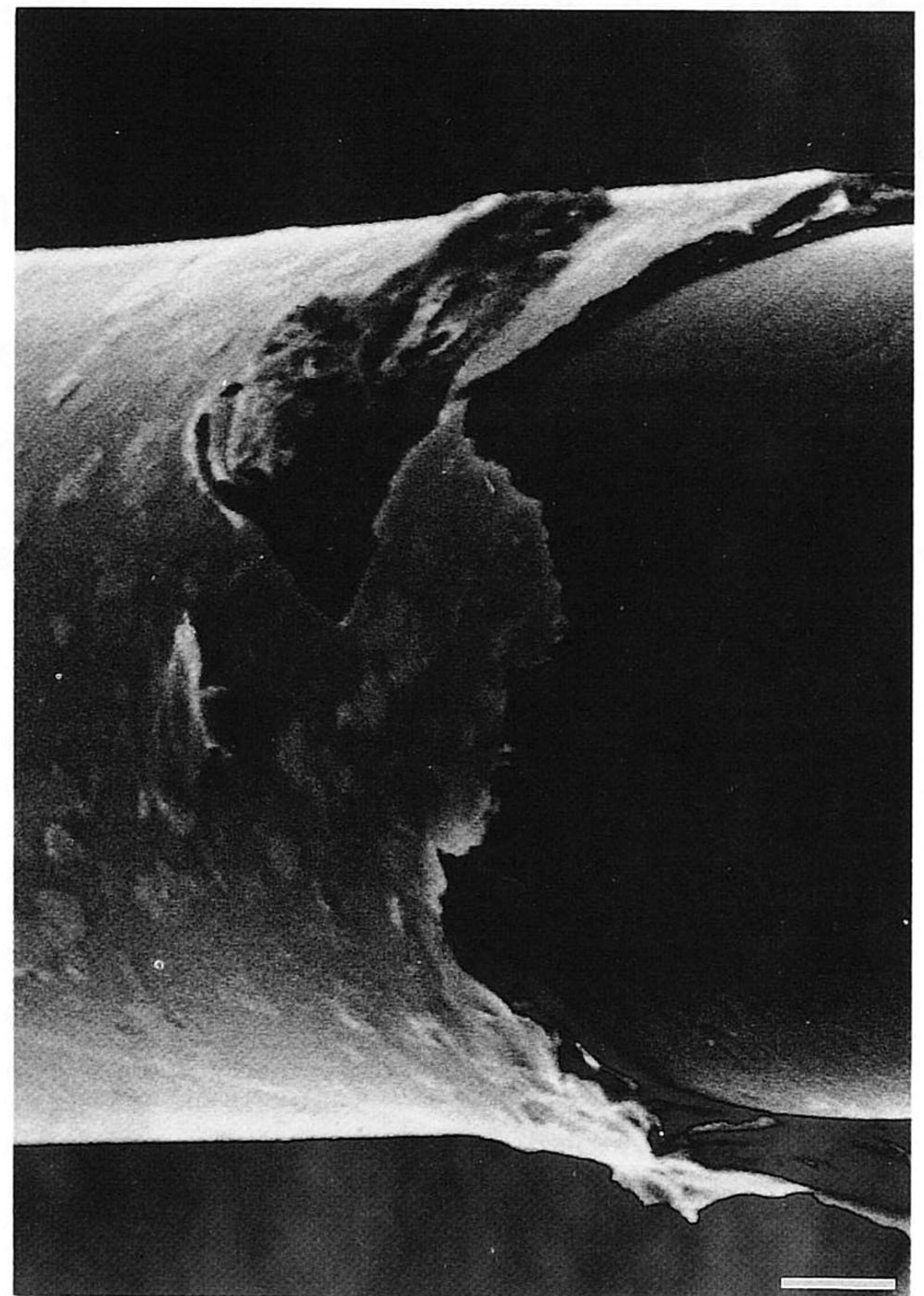
Fig. 2. Scanning electron micrograph of a Biogold-coated Wallstent, showing the thin polymer layer covering the metal wire. Bar = 9 \mu m. Published with permission [11].
