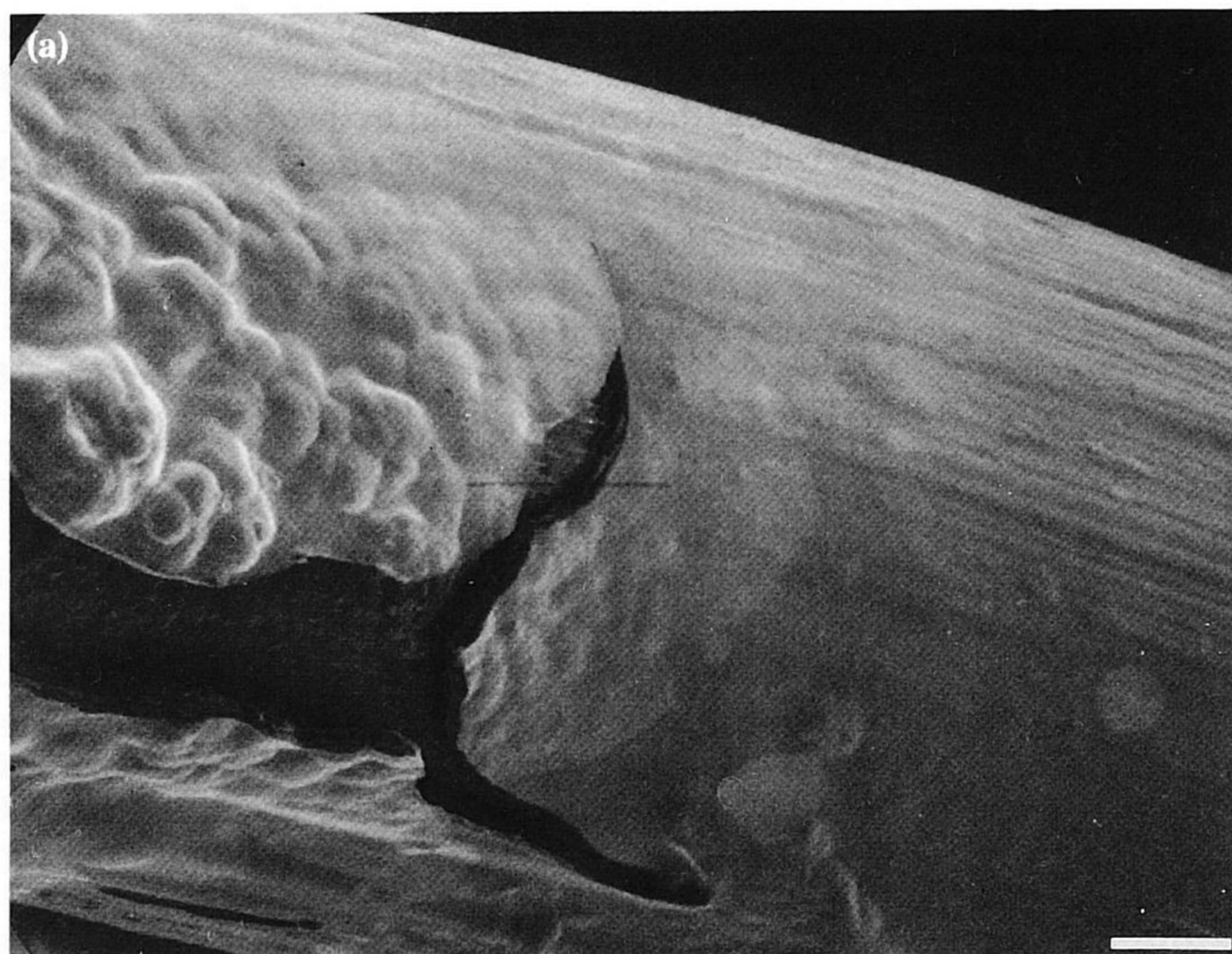
Fig. 4. (a) Scanning electron micrograph of an extracellular matrix-coated Wiktor stent, showing the thin layer covering the metal wire. Bar = 20 \mu m. (b) Light microscopy, 1 week after implantation of an extracellular matrix-coated stent in normal porcine coronary arteries. The extracellular matrix material is covered directly with endothelial and smooth muscle cells, whereas thrombus remnants are not observed. Resorcin-Fuchsin stain. Bar = 30 \mu m.
