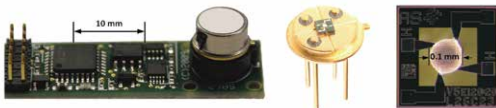
Figure 1.4. The sensor module utilized in the eNose technology of The eNose Company. Left: A sensor module containing the sensor in a metal cap with a white Gore-Tex membrane on top, temperature controlling electronics and microprocessor. Middle: The sensor with cap removed (the white dot is the actual sensor material seen at 100 micron diameter). Right: A close-up of the sensor material with its attached electrodes, 2 opposing electrodes for the heating and the other 2 to measure the resistance.
