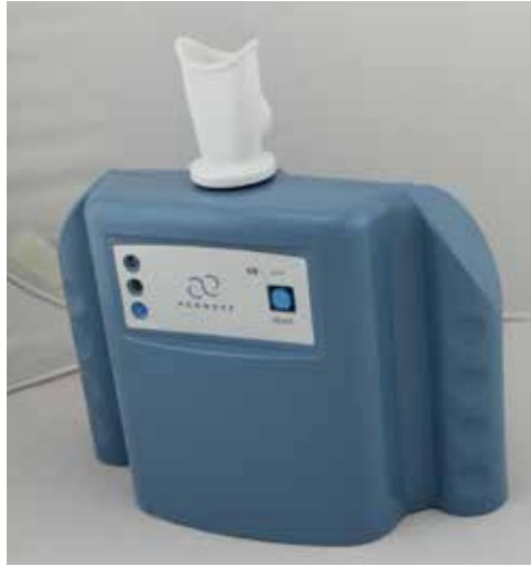
Figure 10.2. The Aeonose, developed for breath analysis
