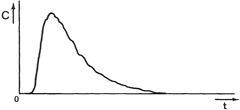
Fig. 1. Outflow concentration of indicator versus time after a bolus injection without recirculation.
