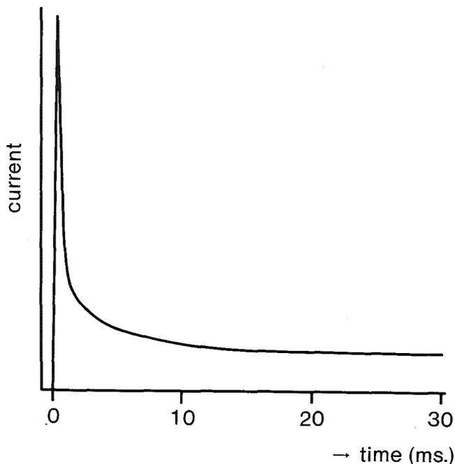
Fig. 2: Time course of diffusion limited current after closing the electric circuit for  $O_2$  polarography.
