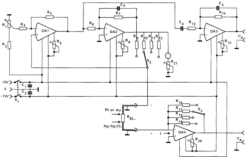
Fig. 7: Electric feedback circuit maintaining a constant polarisation voltage at a desired value. This voltage is measured by operational amplifier OA1. OA2: inverting amplifier; OA3: for AC amplification; OA4:  $O_2/H_2$  amplifier. List of major resistance and capacitance values:
