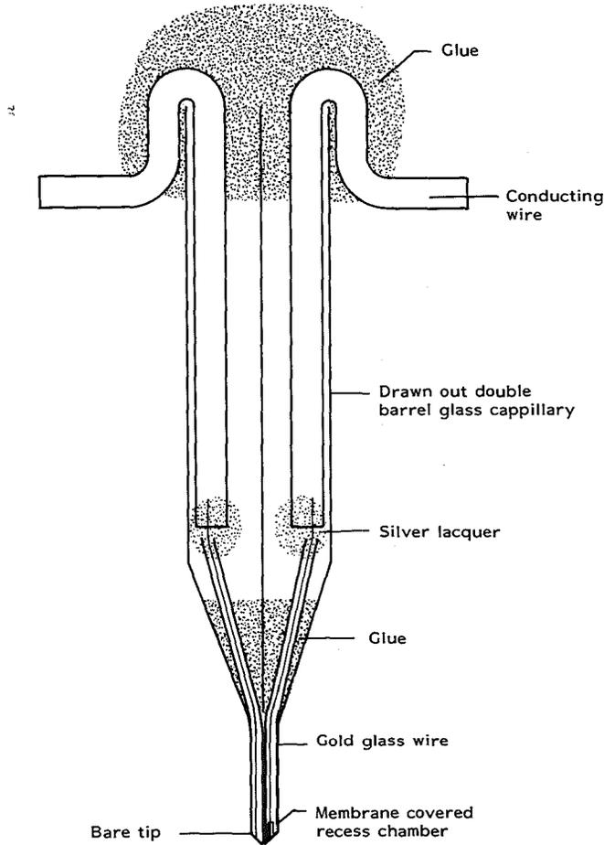
Fig. 5: Double-barrelled microelectrode for  $PO_2$ ,  $O_2$  concentration,  $KO_2$  and  $O_2$ -solubility determination.
