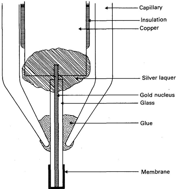
Fig. 3: Oxygen microelectrode.
