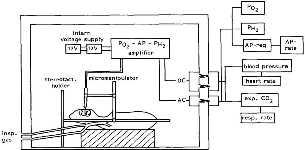
Fig. 8: Experimental procedure in highly shielded cage. The animal is fixed in a stereotactic holder inside a chamber of 2 mm copper surrounded by a chamber of 5 mm steel. The electrode is driven in the tissue by means of a micromanipulator. The signals are outputted via LED's so that no galvanic connection exists between the inside and outside of the cage.
