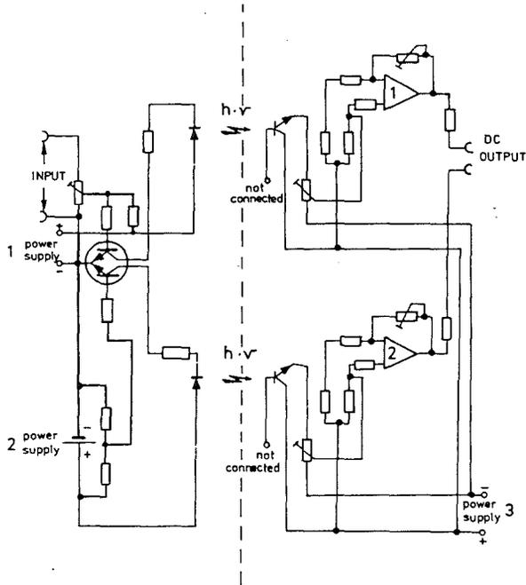
Fig. 9: Diagram of a symmetric two-channel electronic system for DC transmission with automatic temperature correction.
