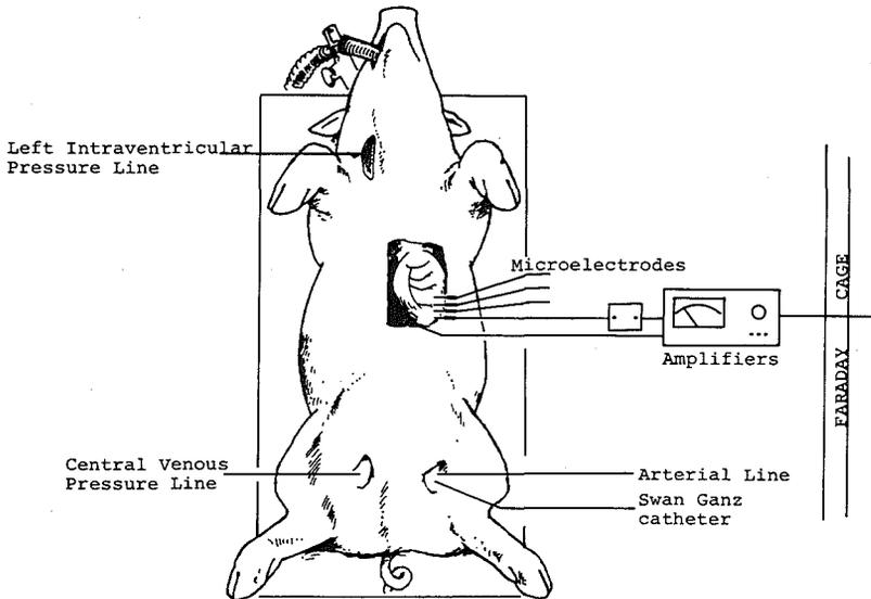
Fig. 1: Experimental arrangement of the animal in the electrically noise-free Faraday cage.
