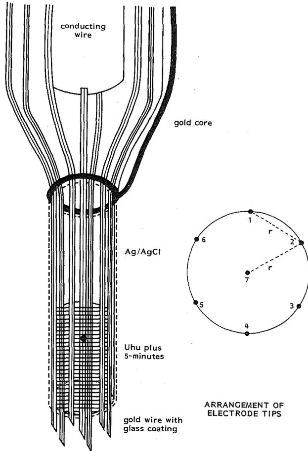
Fig. 4: Diagram of multi-microelectrodes.
