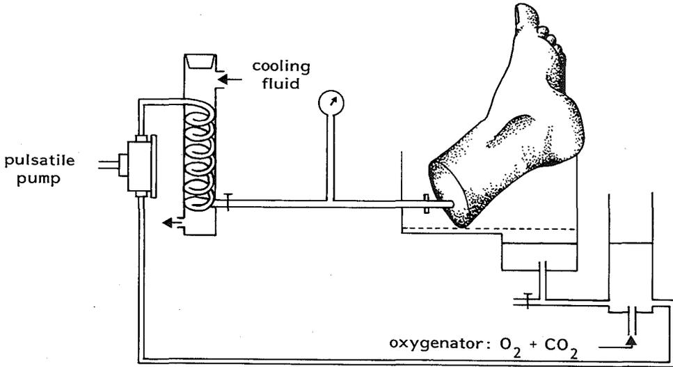
Fig. 6: Experimental setup for perfusing amputated extremities.
