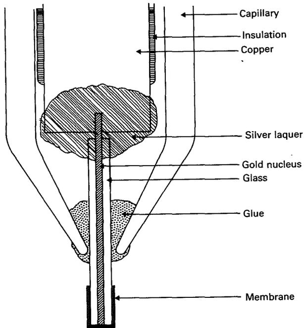
Fig. 2: Oxygen microelectrode.
