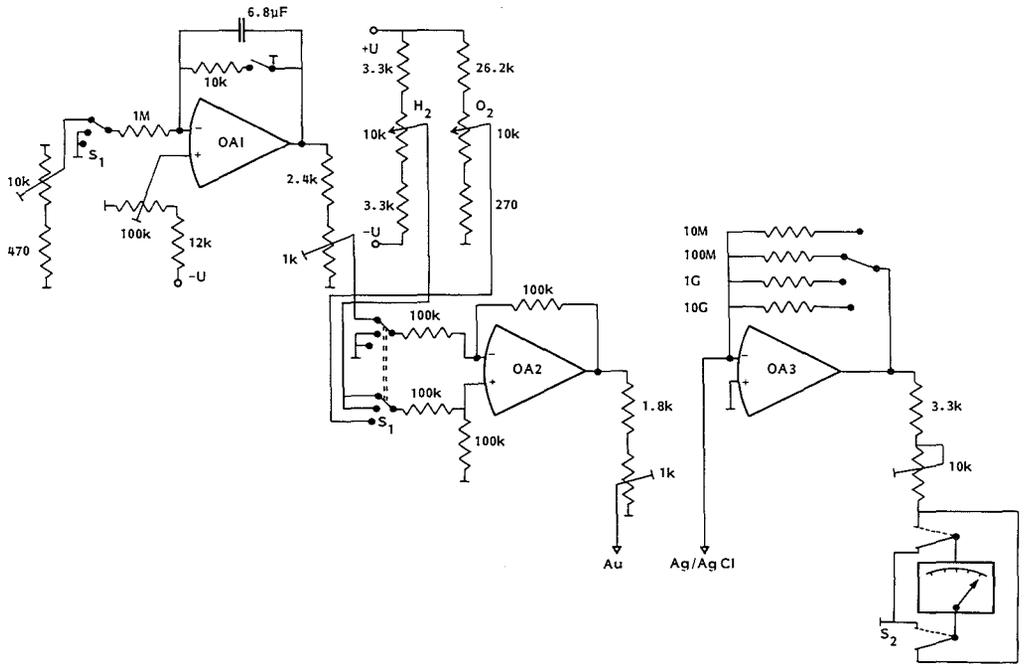
Fig. 6: Diagram of a specified  $H_2-O_2$  measuring system.
