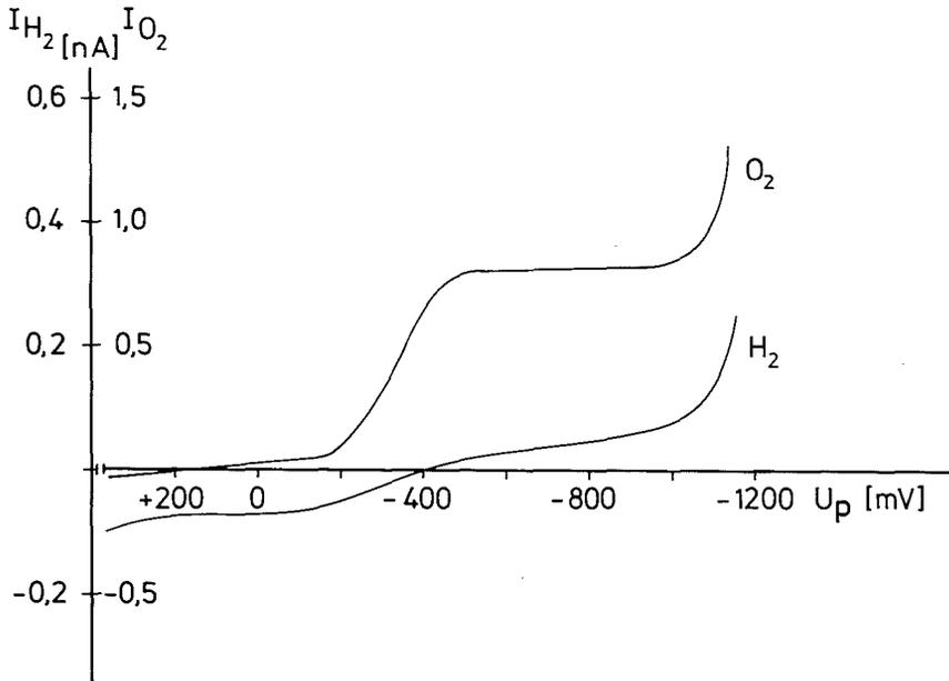
Fig. 1:  $O_2$  and  $H_2$  polarograms of a 10 micron gold electrode. The  $O_2$  curve has a broad plateau between -500 and -1100 mV, the  $H_2$  curve between +200 and -100 mV, and a secondary less characteristic one between -600 and -1000 mV. As the  $O_2$  voltage current curve cuts the base line at about +200 to +100 mV, this would be the voltage range suitable for  $H_2$ -clearance measurements.
