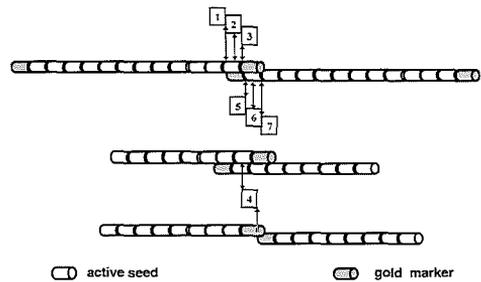
Fig. 1. Points related to the source, in which the dose was calculated.
