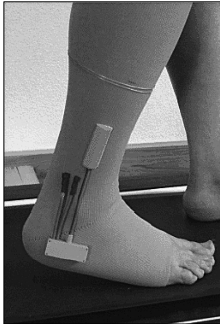
Figure 1 Volunteer with MHC. Registration of the circumference of the leg and the ankle angle.
